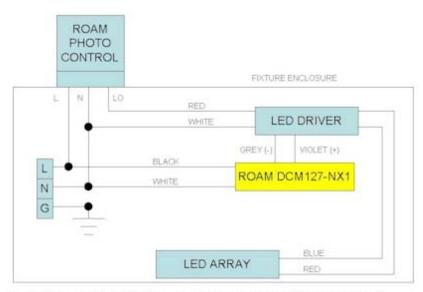
All connections to DCM are provided as flying leads. DCM power is derived from fixture terminal block.
